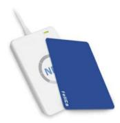
The AC122U NFC Reader is a PC-linked Contactless Smart Card Reader/Writer developed on the 13.56MHz Contactless Technology. It is the world's first CCID Compliant Contactless Card Reader/Writer that follows both ISO14443 and ISO18092. It is designed to support not only MiFare and ISO14443 Type A and B Cards but also FeliCa and NFC tags.
